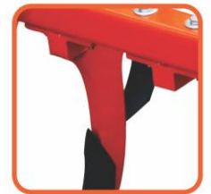
Heavy Duty Profile Cut Tyne
